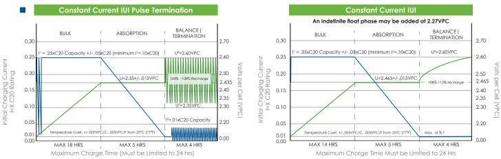
NOTE: This algorithm uses a pulse termination criterion. As a safety precaution during the Finish phase, if the average cell voltage, or volts per cell (vpc), exceeds V2 and the charger output has been on for more than 30 seconds, the output is shut off until the vpc falls to V3. The finish phase then resumes and this "pulsing" continues until the target overcharge (108% - 112%) is reached.
